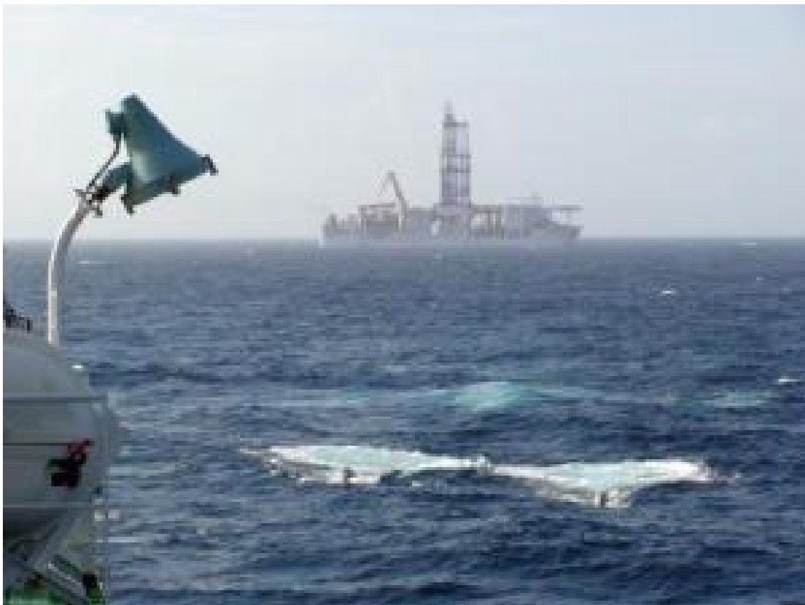
The Japanese research vessel KAIREI shoots air-gun for vertical seismic profiling experiment conducted in the Kimano Basin. (Credit: JAMSTEC/IODP)
