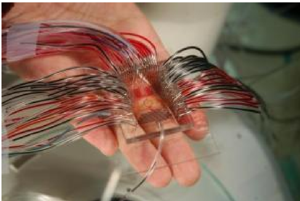
A microfluidic device held in the palm of the hand. (Credit: Image courtesy of University of California - Los Angeles)
